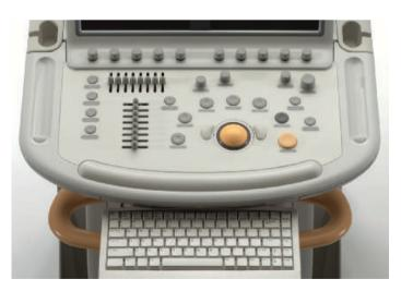
The ergo-centric iE33 control panel places primary keys for easy accessibility. It features tri-state lighting to help you while scanning in dark environments.
