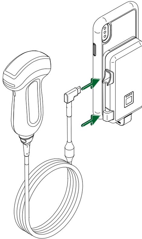
Connecting the Transducer Cable to the LPM
